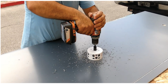
*Cutting valve hole with hole saw
