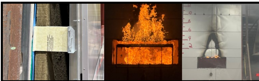
Figure 1: ALUCOBOND® PLUS Before, During and After NFPA 285 Testing with 7" Cavity Air Gap
