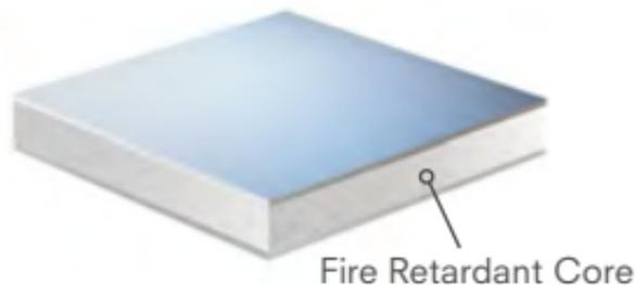
4mm aluminum composite material (ACM) comprised of two sheets of smooth .020" aluminum thermobonded to a solid, fire retardant core. Developed exclusively to meet fire performance requirements while providing the benefits & versatility of ACM.
