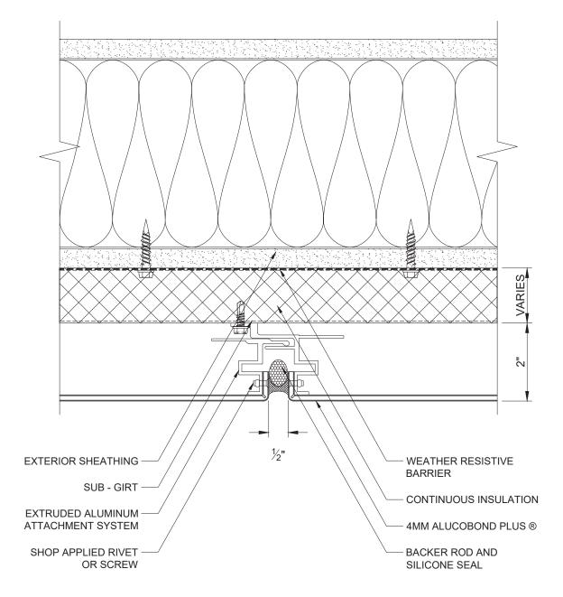
VERTICAL JOINT - PLAN VIEW SCALE: 3" = 1' - 0"
