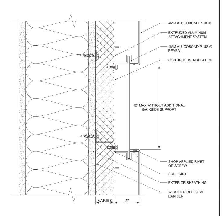
EXPANDED REVEAL JOINT SCALE: 3" = 1' - 0"
