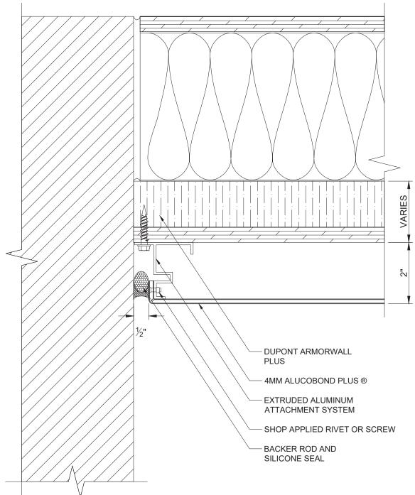
507 END WALL - PLAN VIEW SCALE: 3" = 1' - 0"
