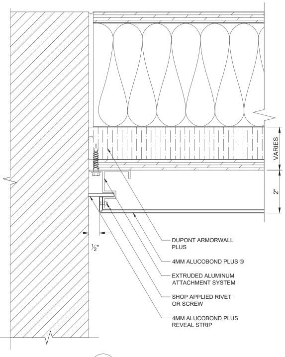
507 END WALL - PLAN VIEW SCALE: 3" = 1' - 0"
